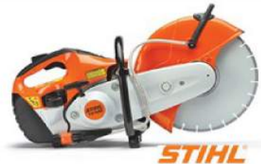
14" Gas Cutquik Saw 4.9" cut depth, X2 air filtration system, 24-oz. fuel capacity (TS420)
